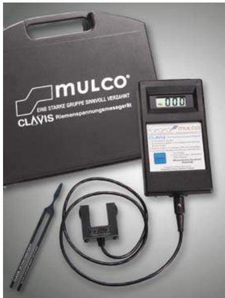
**Clavis uses microphones to acoustically measure the frequency of the vibrating belt.**
